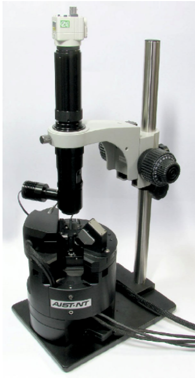
Fig. 2. Photograph of the SMART-SPM 1000 atomic force microscope that was used in the experiments.
