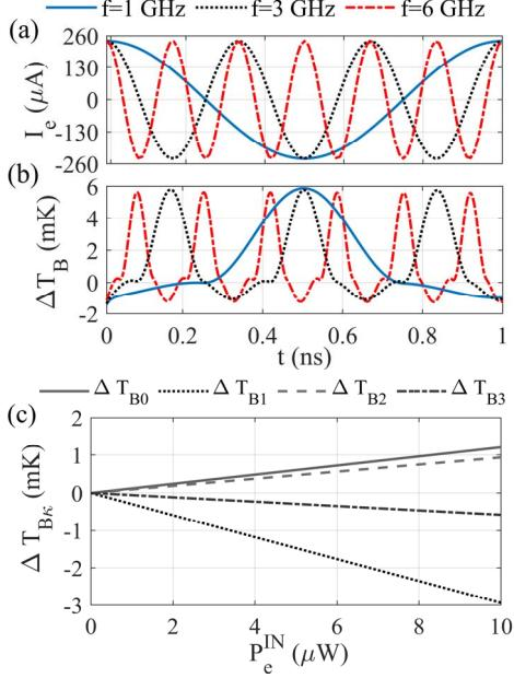
Fig. 2. (a) Time evolution of (a) the microwave current and (b) the temperature drop  $\Delta T_B(\omega)$  across the tunnel barrier of MTJ at different frequencies (color online). (c) Dependence of the magnitude of the  $\kappa$ -th harmonic  $\Delta T_{B\kappa}$  of the temperature drop on the heating power.
