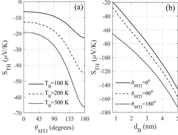
Fig. 4. The frequency-independent Seebeck coefficient  $S_{TH}$  as a function of (a) the angle  $\theta_{MTJ}$  between  $\mathbf{m}$  and  $\mathbf{m}_p$  and (b) the height  $d_B$  of the tunnel barrier of the CoFeB-MgO-CoFeB MTJ.
