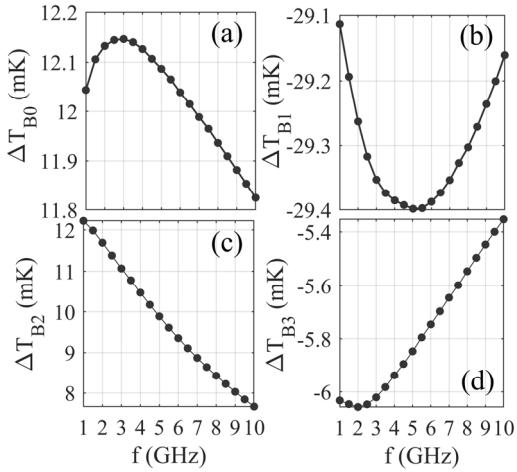
Fig. 3. The dependence of the amplitudes of  $\kappa$ -th harmonics (a)  $\Delta T_{B0}$ , (b)  $\Delta T_{B1}$ , (c)  $\Delta T_{B2}$  and (d)  $\Delta T_{B3}$  on frequency at the input microwave power of 10  $\mu\text{W}$ .
