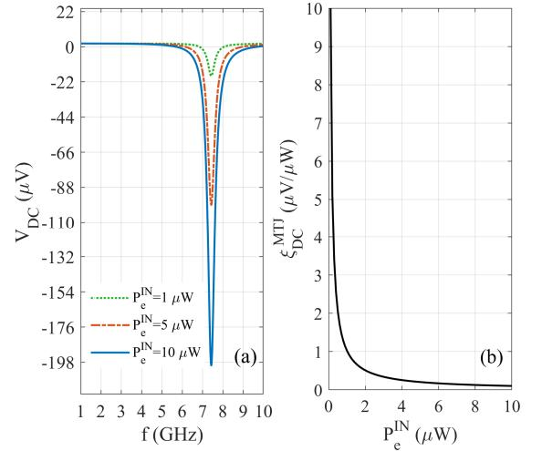
Fig. 5. (a) The frequency dependence of the d.c. voltage  $V_{DC}$  for varied input microwave power at a temperature of 300K (color online). (b) Dependence of the thermal contribution to microwave sensitivity  $\xi_{DC}^{MTJ}$  of the spin-torque diode on the microwave input power at the a.c. current frequency of 10 GHz. The magnetic field  $B$  is equal to 50 mT and the parameters of MTJ were taken from [14, 20].
