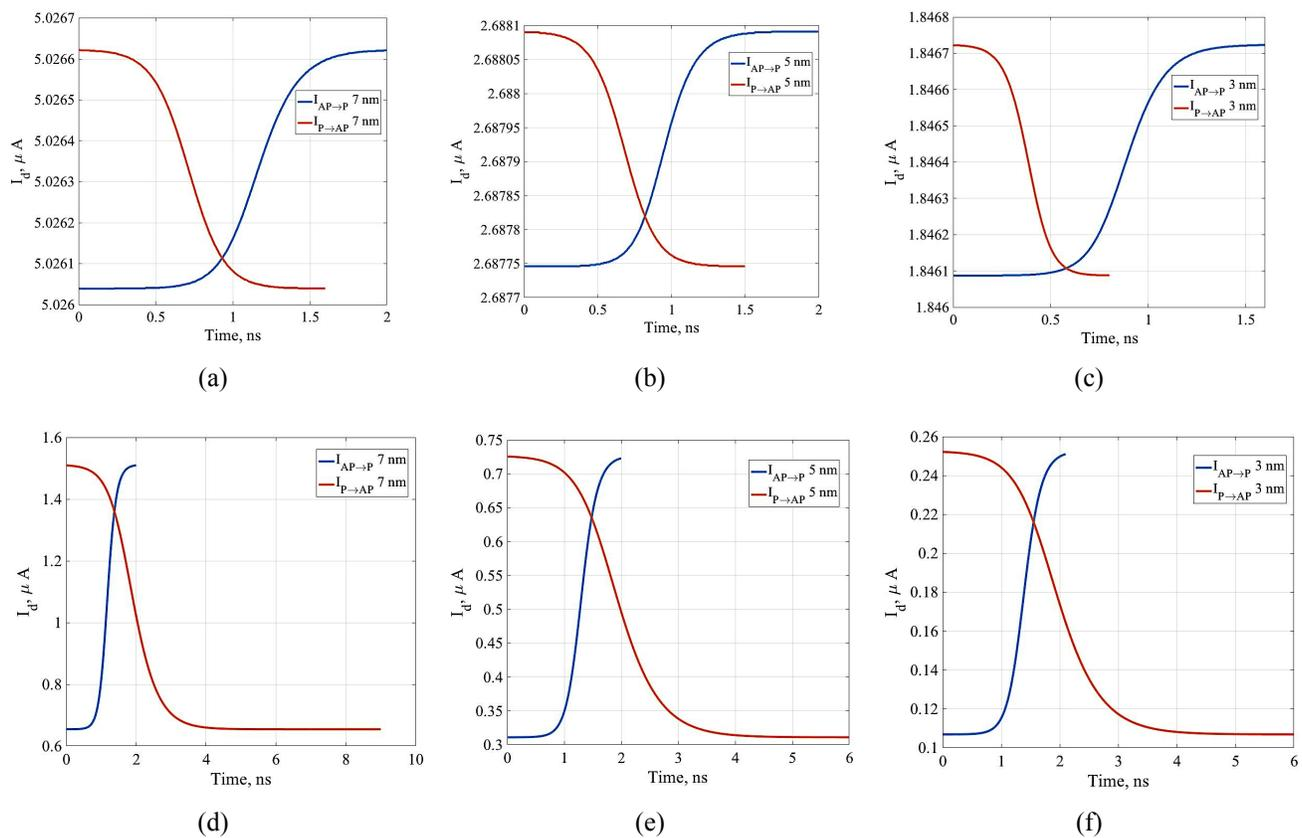
Figure 7. Switching characteristics of the current when switching the STT-MRAM cell for various technology nodes: for the magnetic nanobridge (a-c) and for the MTJ (d-f)
