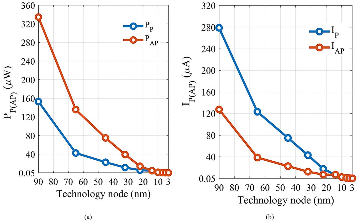
Figure 6. (a) Power consumption and (b) averaged current for switching the magnetoresistive cell of STT-MRAM from P (AP) to AP (P) state, depending from the technology node.
