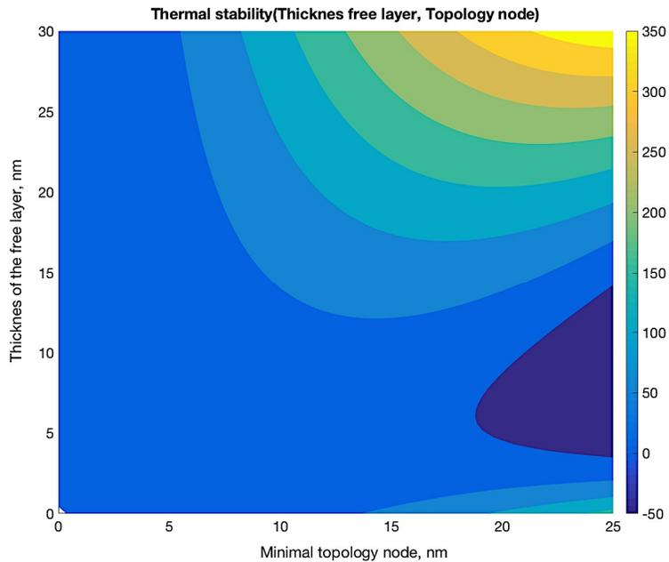
Figure 8. The diagram of thermal stability of MTJ depending on the thickness of the free layer and minimal topology node equal to the diameter of MTJ.
