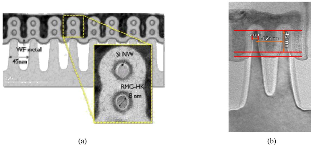
Figure 4. (a) NW GAA FET from Imec with the topology of 8 nm (2016) and (b) FinFET from Intel with a topology of 14 nm [13, 14].
