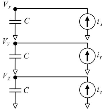
Figure 2. The equivalent circuit for the integration of the LLGS equation in HSPICE model of the magnetoresistive memory cell of STT-MRAM.
