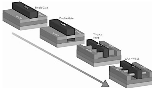
Figure 3. The evolution of the transistor from planar MOSFET to bulk GAA FET.
